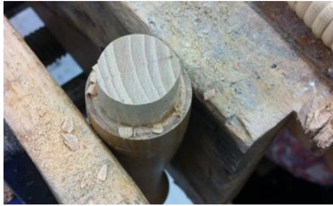
Figure 91 – Hand chiselling on the back of the hook to fit the hole
