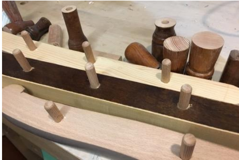
Figure 93 – 10mm dowel drilling and fixing on the body of the coatrack and hooks
