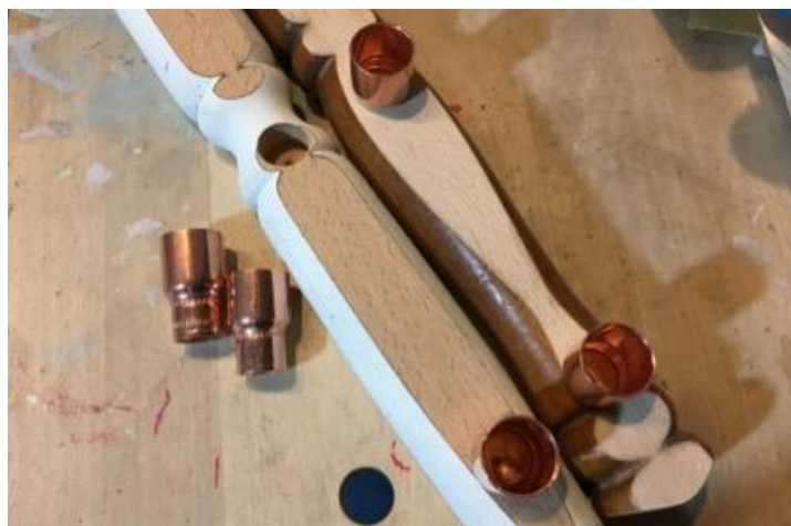
Figure 116 – Copper end-reducer for the candle insert that comfortably fits existing hardware for its new purpose
