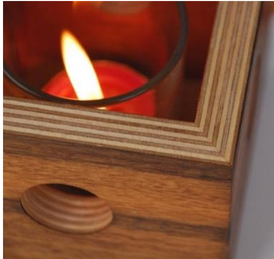
Figure 55 – Mitred Ply Box Tea Light Holder, made of plywood from an old G-Plan sewing cabinet. The boxes have been mitred together at the corners to go with the flow of the ply.
