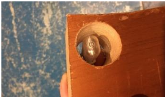
Figure 112 – Space of at least 30mm needed to change the G9 bulb
