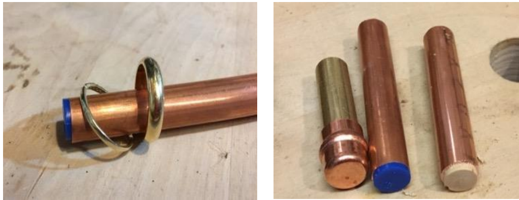
Figure 126 – Copper tube and brass rod in working progress (left), finding right diameter for rings (right) test for an end finish
