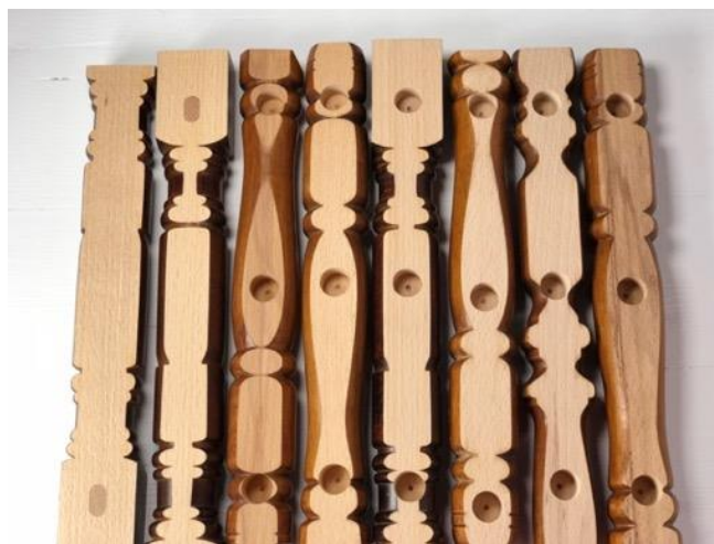
Figure 118 – Holes made by 18mm Forstner bit to hold candle cups
