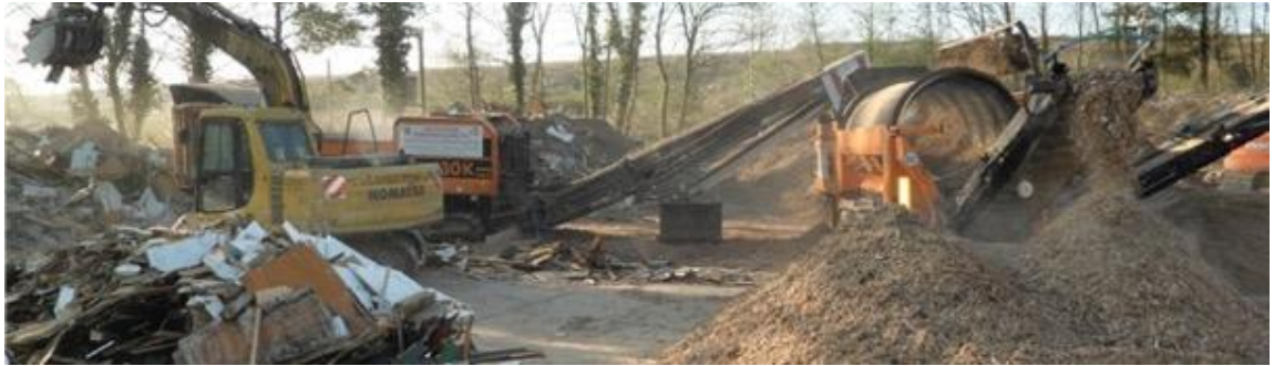
Figure 13 – Once the wood has been collected or tipped it is separated then put through a shredder. It is then screened to produce different grades of wood chips. The larger woodchips are mainly sent to chipboard factories, while the finer material is used for cattle bedding © South Wales Wood Recycling.
