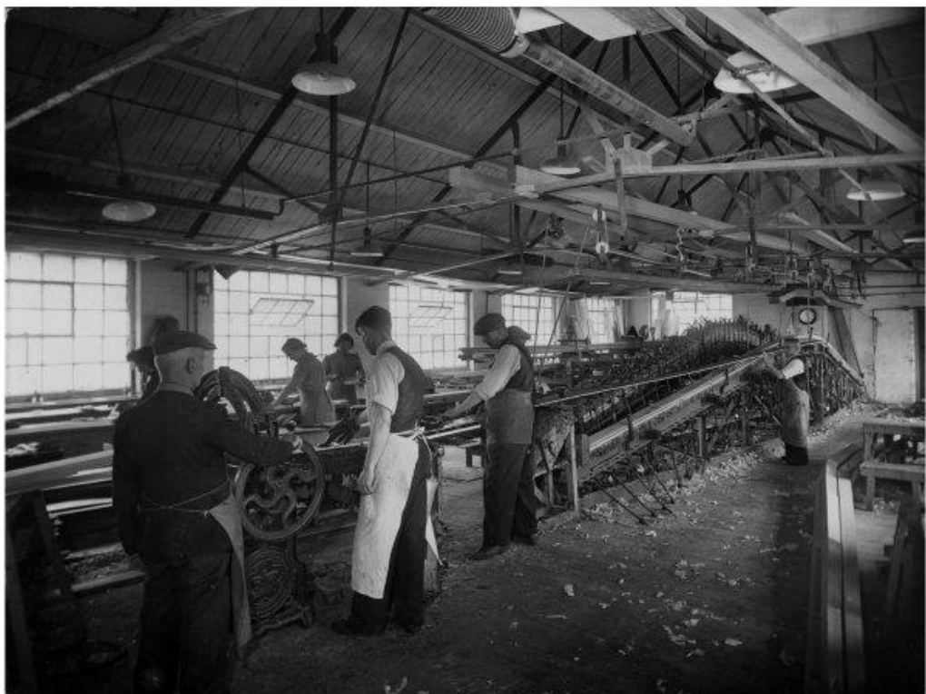
Figure 172 Gluing of wing spar plies for De Havilland Mosquito aircraft at J.B. Heath (Heathland) Furniture Ltd, High Wycombe, c.1942-45
