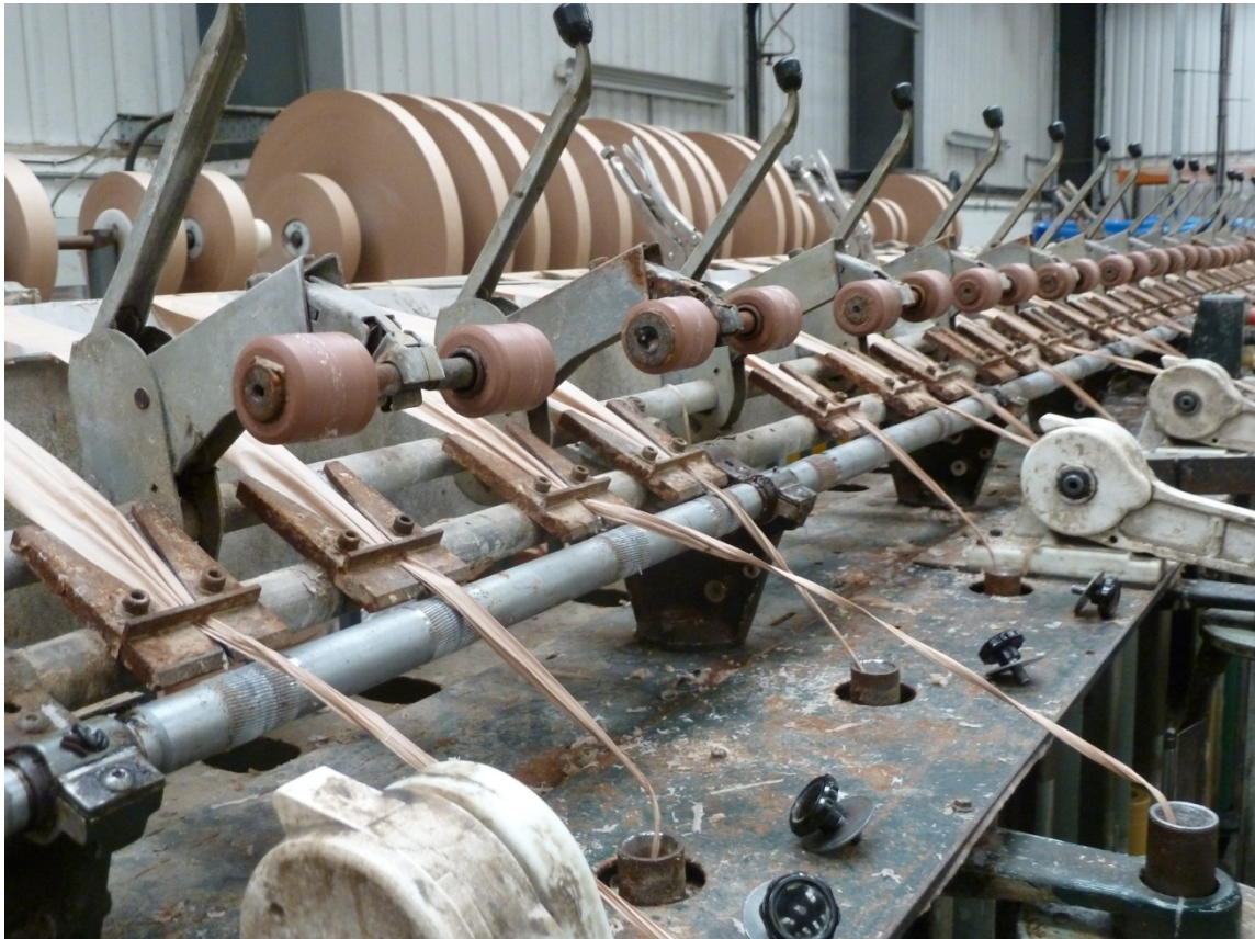
Figure 5: Woven paper manufacture at Lloyd Loom, Spalding, UK
