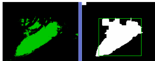
Figure 5-16 (a): Full opened eye sclera region, image from left- (i) captured eye sclera image using green illumination system, (ii) Blob analysis tracking image.
