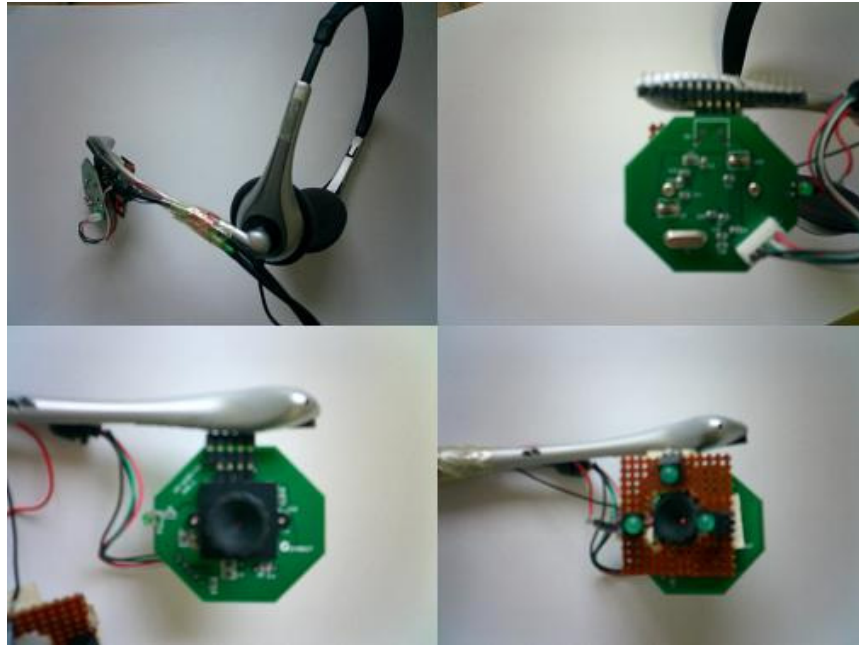
Figure 5-1: Prototype system of Eye blink capture device
