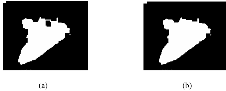
Figure 5-15: (a) Binary image before adding morphological Closing, (b) after morphological Closing
