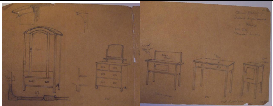
Fig. 2-115. A.H.'s original pencil sketch for the sanatorium furniture. Note detail of curved interior corner to wardrobe to avoid dust trap. Interiors were also to be polished, wash stand and pedestal to have opal glass tops, handles to be gunmetal, finish was to be mahogany colour. (H&S Archive AAD/1994/16/824)
