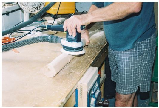
Fig 9. Sanding reeds using an electrical orbital sander
