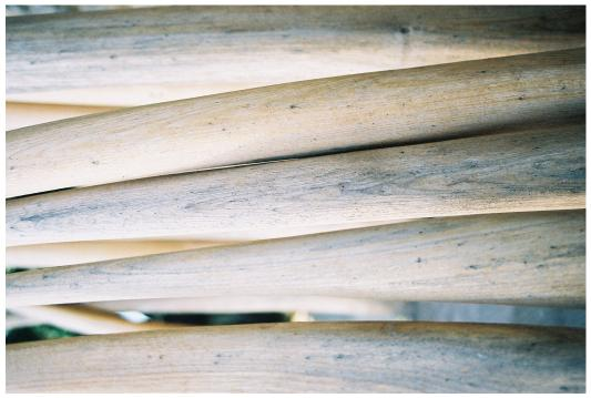
Fig 14c. Detail of finish after fourteen months revealing slight tannin staining after exposure
