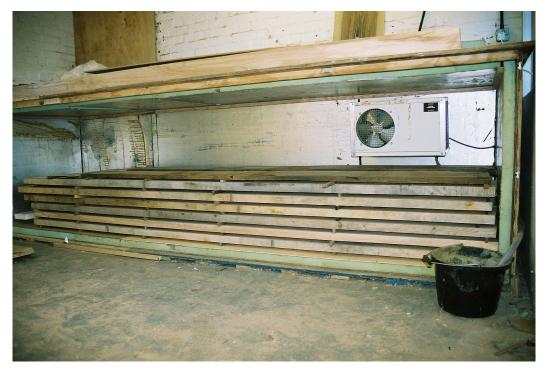
Fig 39. Dehumidifier unit set up in the Philip Koomen Furniture workshop where the air-dried timber from the workshop yard is dried between 8–12 per cent moisture content, ready for construction. This photo shows 50 mm ash from Cookley Green, Oxfordshire, and 30 mm brown oak from Thame Park, Oxfordshire
