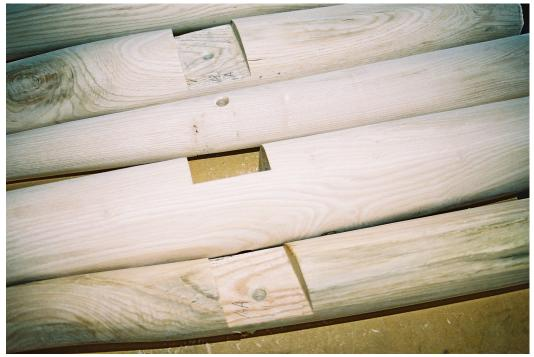
Fig 11. Housing joints are cut
