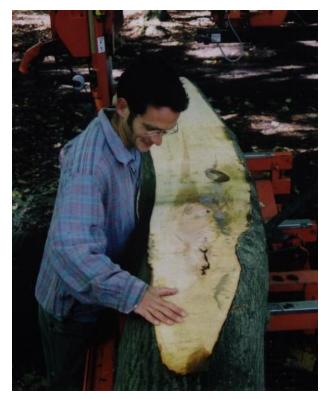
Fig 30a. First cut on the mobile Woodmizer sawmill
