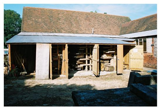
Fig 38b. Air-dried boards are stacked in the purpose made timber store until they can be dried in the workshop dehumidifier unit
