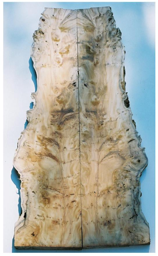
Fig 64. Two book-matched pippy yew boards, from Christmas Common, feature convoluted waney edges. This provides the form for a plank table
