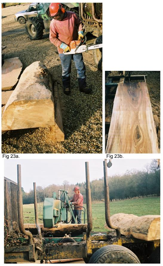
Fig 23c.Fig 23 a/b/c. Conversion of olive ash logs at StonorPark using a Forestor
