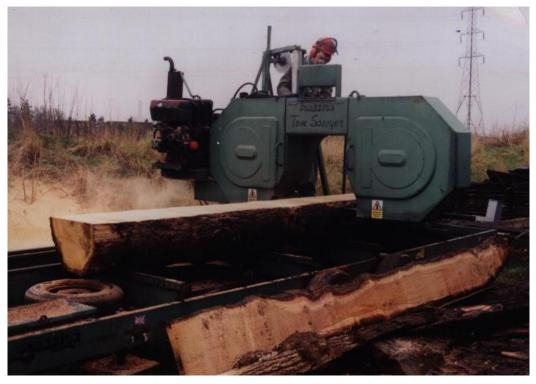
Fig 32a. The catspaw oak log being sawn by Martin Drew using a Forestor mobile saw
