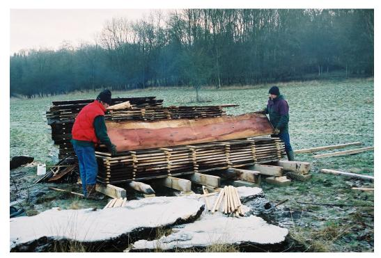
Fig 26a. Stacking boards ready for air-drying
