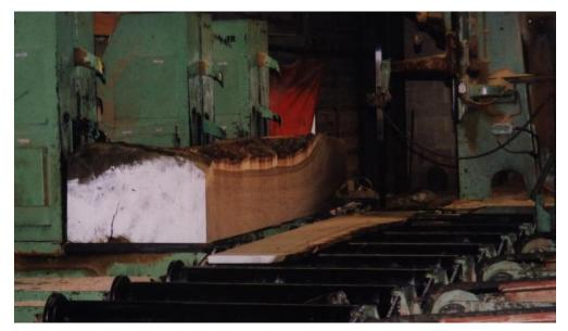
Fig 34a. An individual sawmill at work; removing the first plank of brown oak
