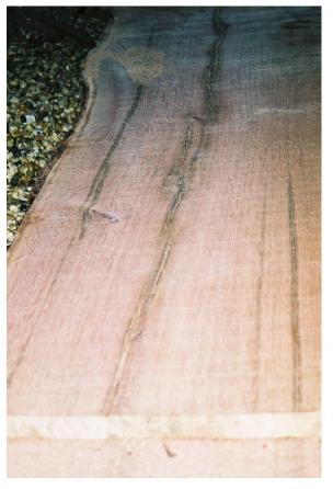
Fig 25b. One of the logs showing cracks distinguished by the stains
