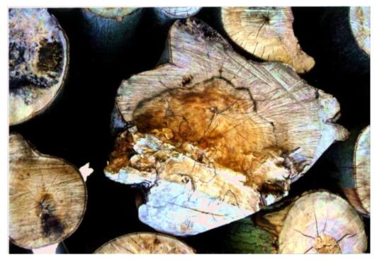
Fig 54a. A spalted beech log
