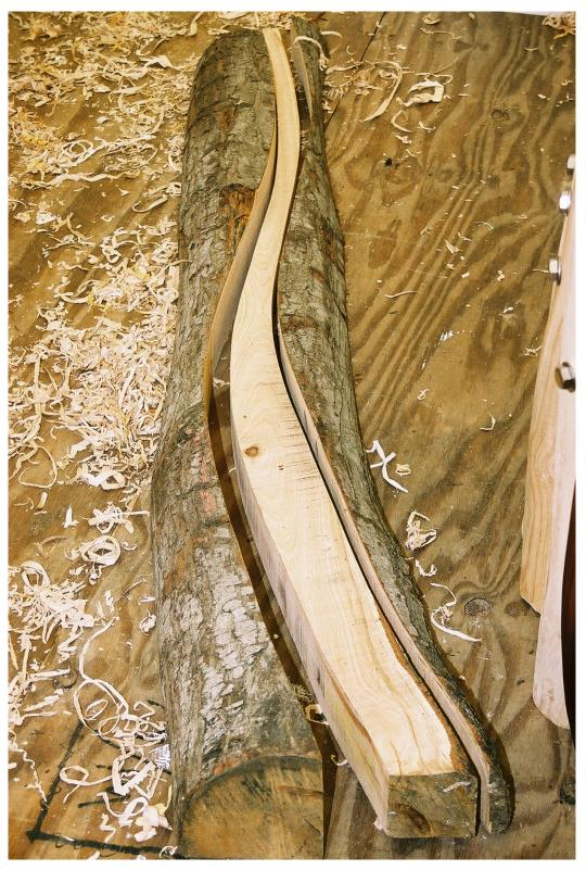
Fig 67. Forming the reeds for "Pondlife" benches. Each reed follows the natural curve of each sweet chestnut thinning
