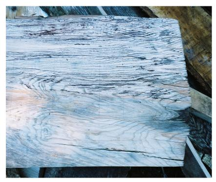
Fig 37. Ash board revealing advanced decay after being left in the round for too long
