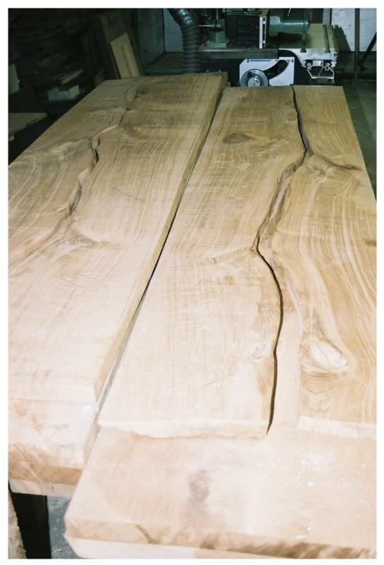
Fig 46. Original two book-matched tiger oak boards showing the contours of the split before re-sawing
