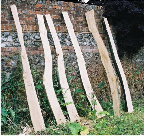
Fig 3. Split logs ready for band sawing
