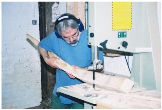
Fig 6. The sections are reshaped into octagonal sections
