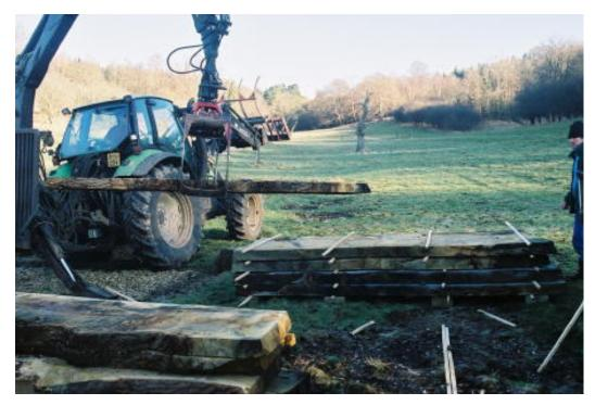
Fig 24b. 100 mm thick boards being stacked to air-dry at the estate
