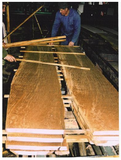
Fig 34b. Sawn planks of brown oak: "stickers" being positioned ready for drying
