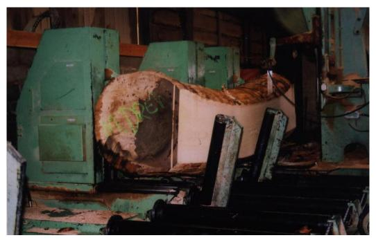
Fig 42a. An ash log being sawn at Helmdon Sawmill. The outer boards produce white boards
