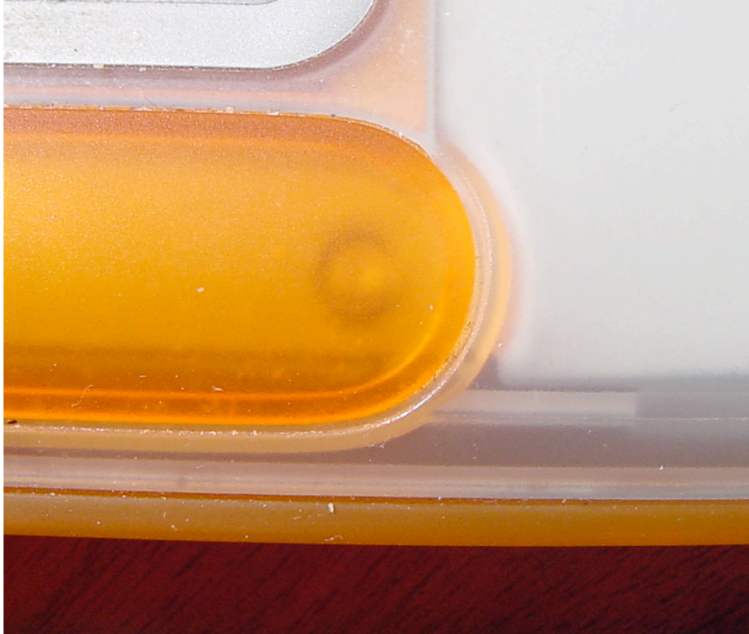
fig. 26 The visible 'dots' which sit at the centre of the space formed by the semicircles at the curved ends of the 'click' bar.
