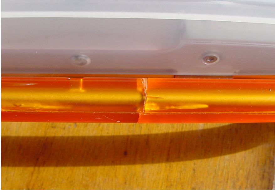
fig. 35 The cracked handle...
